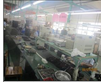
Photo of non-conformity NC 7.25 No local ventilation facility was equipped for the soldering positions of the repairing area.JPG
